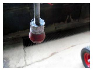
Next I did some sanding and filing to shape the JB Weld part back into the bottom of the knob.
