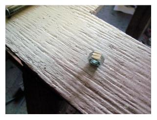
Next I threaded the nut onto a 3/8" UNC bolt after I applied a light coating of grease to the threads on the bolt. Then I threaded the remaining top of the shiter knob onto the bolt and made a collar out of cardboard and masking tape and placed the collar around the nut. After the collar was taped to the knob I hung the knob upside down and filled the collar with JB Weld.
