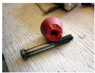
Since the shifter lever was 3/8" UNC thread I got a 3/8" UNC nut and cut a few grooves in the hex part of it with a hack saw to give the JB Weld something to bond to – a file could be also be used to get similar results.
